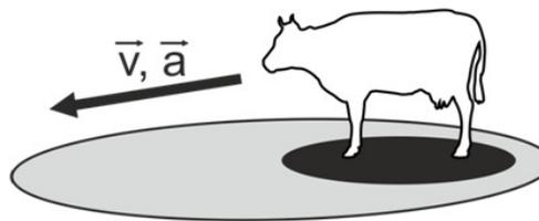
Fig. 3. Moving obstacle with dynamically changing virtual influence zone
